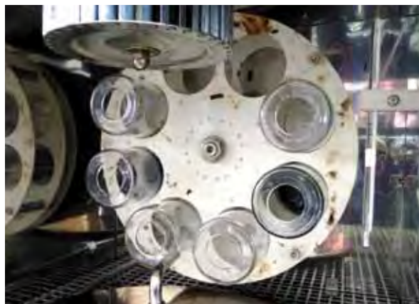
Figure 2.25. View of glass containers for bitumen samples (A) and containers installed in the RTFOT drier (B) (photo by ORLEN Asphalt sp. z o.o., courtesy of ORLEN Laboratorium sp. z o.o.)
