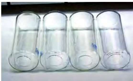
Figure 2.25. View of glass containers for bitumen samples (A) and containers installed in the RTFOT drier (B) (photo by ORLEN Asphalt sp. z o.o., courtesy of ORLEN Laboratorium sp. z o.o.)
